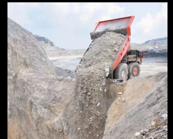
Dumping into the vertical shaft
